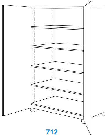
712 Storage w/ Doors Diaphragm bottom required
